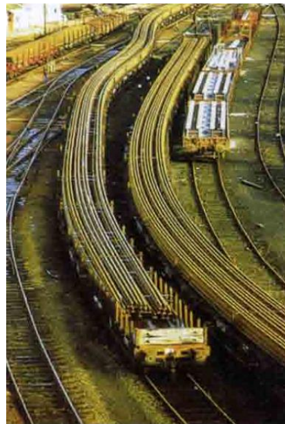
Fig. 1. Transportation of rail lashes to the installation site
